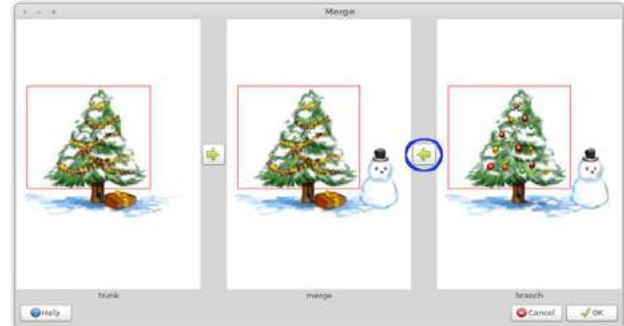
Figure 5: UI for revision merging. (a) shows the merge UI. Images at left and right are revisions to be merged while the center is the preview of the merge result. (b) is the automatic merge result. Non-conflict edits (gift and snowman) are automatically merged while for conflict ones (ornamental strips and balls) the trunk version is chosen by default. Our system also allows users to change the default behavior, including branch-after-trunk (c) by clicking the blue circled button once, branch-only (d) by clicking the blue circled button twice, and trunk-after-branch.
