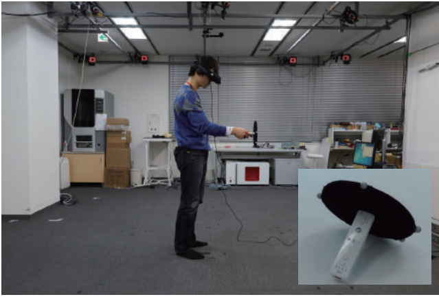
Figure 3: A user wearing an HMD and holding a 6 DoF controller. Both the HMD and controller have additional optical markers attached, and their 3D positions and orientations are tracked with a mocap system.
