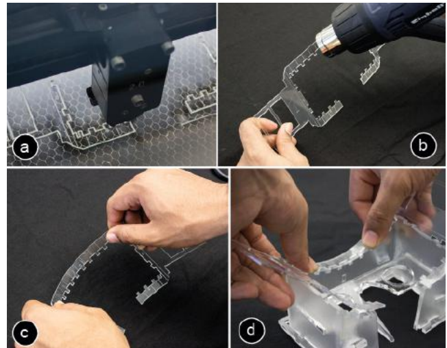
Figure 5: Creating a curved plate from acrylic: (a) cut plate, (b) heat it using a heat gun, (c) pre-curve it, and (d) press it into position to give it the right shape.
