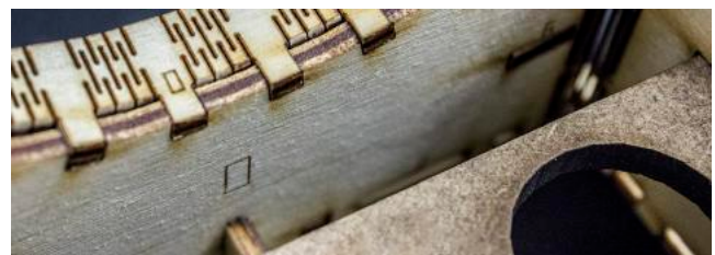
Figure 7: Platener 3D prints/engraves instructions.
