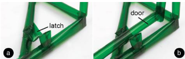
Figure 29: (a) Door latch in the shape of an “M”. The door’s weight allows it to latch into the “M”.
