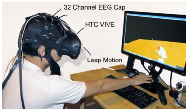
FIGURE 1. Our EEG-based experiment evaluated the interaction techniques in VR by measuring intentionally elicited cognitive conflict.
